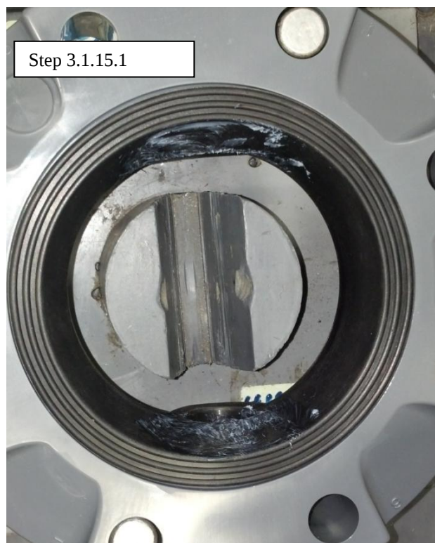
Top of Liner with Counter Bore (3.1.14.1)
