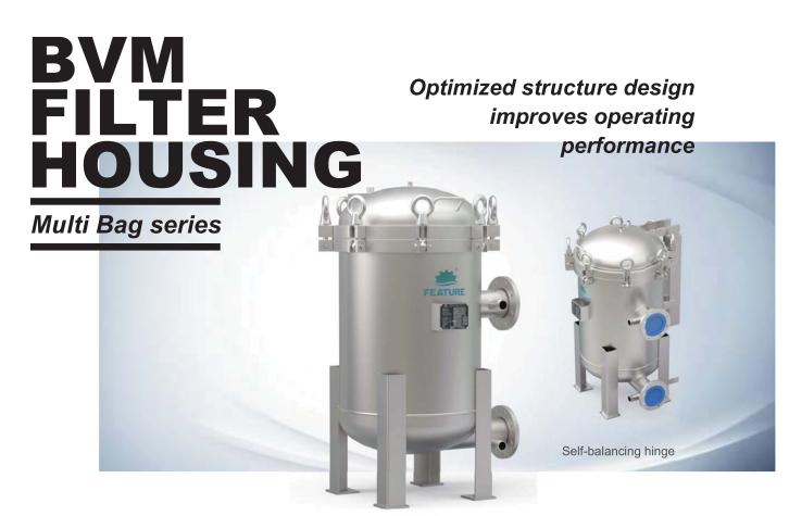
Feature -Tec's BVM multi-bag filter housings features side inlet and bottom outlet, providing easy and complete drainage. The convenient tangential bottom outlet reduces housing height, making bag change-out easy and safe. A standard eye-bolt closure is equipped with Feature-Tec's self-balancing head lifting system for quick access to the interior. Inside, Feature-Tec's unique 3-point bag seal clamp assures bypass-free performance under any conditions.
